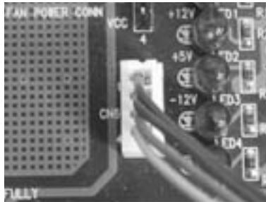
*Figure 5-1. ATX power control connection on backplane*
