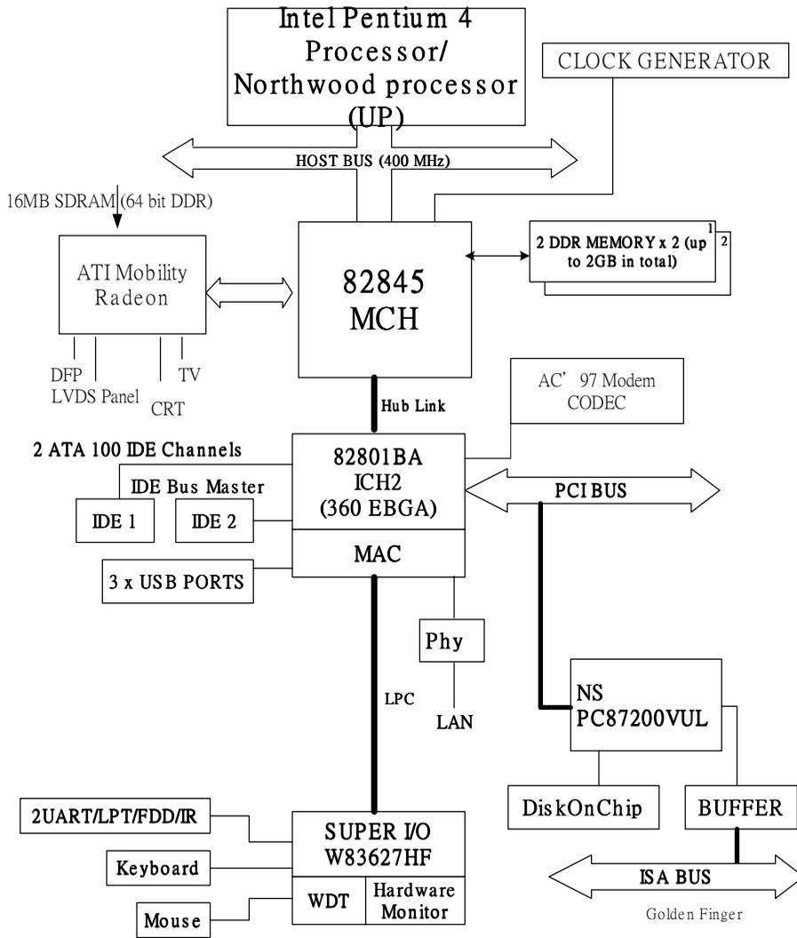
Figure 1-1. SBC-845D-VEA Block Diagram
